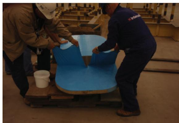
Intergard® 5400 is designed to provide protection to coated substrates and certain non ferrous substrates against incidental surface contamination such as dust, oil, grease, fly-rust and overspray in combination with a degree of resistance to abrasion and scuffing.
