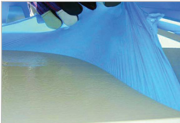
Intergard® 5400 utilizes patented, peelable technology, carefully formulated to ensure easy and complete removal at a wide range of temperatures without deterioration of the underlying substrate.
