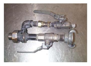
Pressure pot equipment is recommended with bottom paint delivery to the gun, as this reduces the risk of paint blockages. A working pressure gauge and pressure adjustment mechanism is essential.
