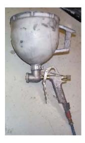
Available air pressure and capacity for spray equipment should be at least 80 psi and 50 cfm (5.5kg/cm<sup>2</sup> and 1.4m<sup>3</sup>/min).
