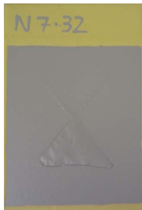
Detachment of topcoat following use of unapproved pen
