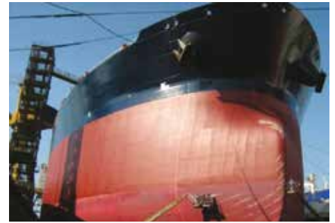
In-dock condition after HPFWW
