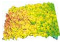
Typical roughness 200-255µm
