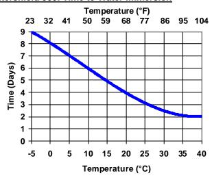
Water immersion refers to water testing to highlight any "holidays" in the coating or ballasting of tanks during sea trials and usually will not exceed 7 days. On deballasting, the tanks must be dried out.
