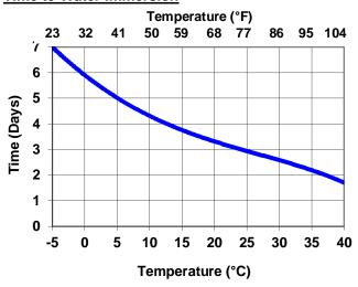
Water immersion refers to water testing to highlight any "holidays" in the coating or ballasting of tanks during sea trials and usually will not exceed 7 days. On deballasting, the tanks must be dried out.
