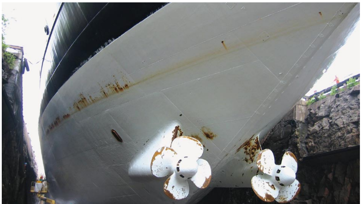
Intershield® 163 Inerta 160 after 60 months in service.
