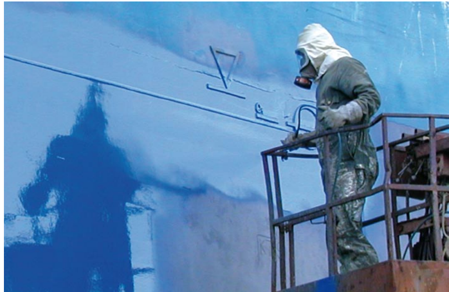
The first Classification Society recognised abrasion resistant ice coating was Intershield® 163 Inerta 160, from International Paint.
