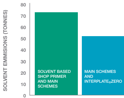
A 130,000 CGT Cruise vessel gives an approximate 25% VOC reduction
