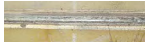
Upper and lower side shows excellent weldability results from submerged arc butt welding
