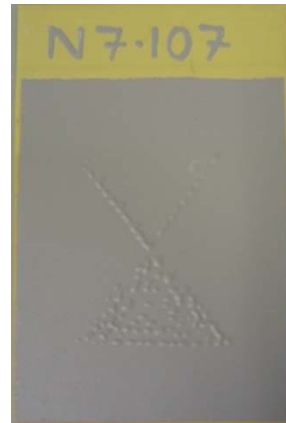
Blistering of topcoat following use of unapproved pen
