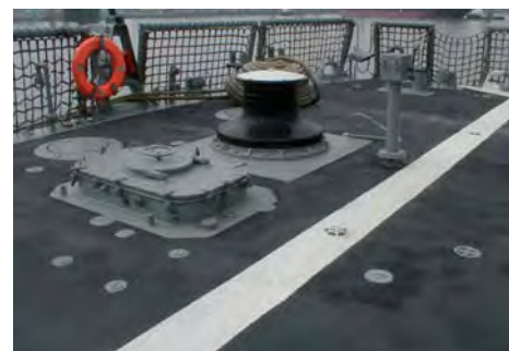
Excellent in service performance providing a safe non skid surface
