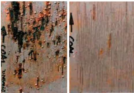
Panels show excellent anti-abrasive properties using an in-house test method, developed in association with the Newcastle University which simulates realistic in-service conditions. Coatings tested with coal cargo at 31,000 kg/m<sup>2</sup>, followed by 18 months immersion in seawater.
