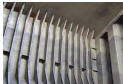
Remarkable resistance to damage in cargo holds after 7.5 years in-service
