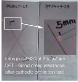
Suitable for use with controlled cathodic protection
