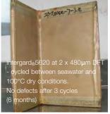
Crack resistance at high film thickness\*
