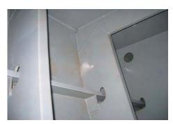
Excellent performance in water ballast tanks of a 3,100 TEU container vessel after 5 years in service
