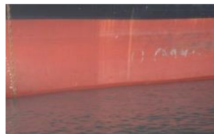
Test patch applied to a 7,120 DWT General Cargo vessel. Trading Korea-China-Japan, high risk coastal fouling challenge
