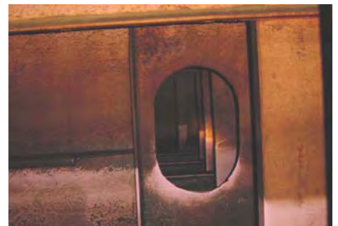
Wing tank - excellent condition after 48 months
