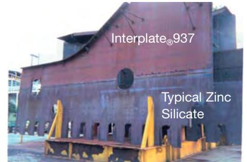
Interplate®937 reduces burn damage and white rust formation compared to typical zinc silicate shop primers
