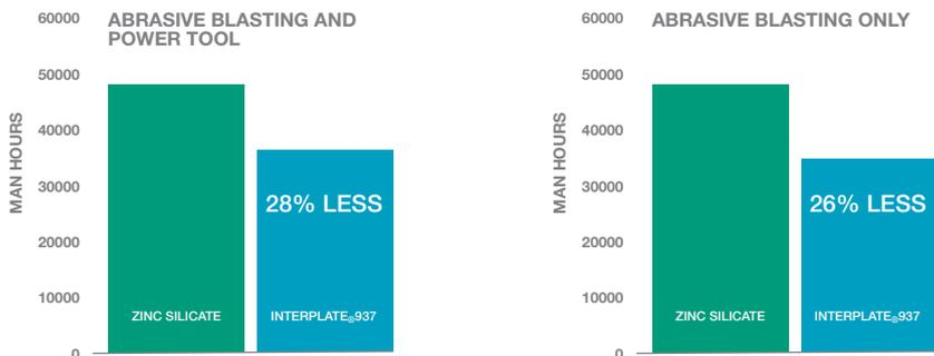
Diagram illustrates the reduction of secondary surface preparation man hours for a 60,000 DWT crude oil tanker when compared to typical zinc silicates.
