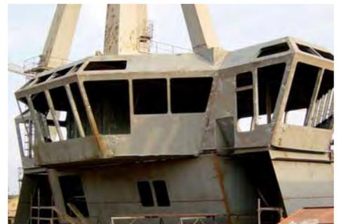
Minimal burn / mechanical damage and white rust even after block fabrication
