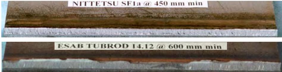
Results from in-house fillet welding test. Interplate®937 shows excellent welding properties using typical welding consumables and welding speeds.
