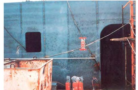
Interplate®937 minimises burn damage on the back of welds
