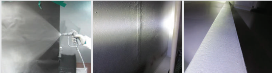
Poor sprayability (shown as above) results in dust over surrounding area and will reduce the gloss of the surfaces.
