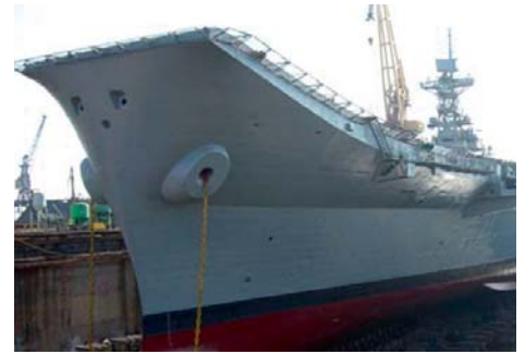
Interlac®1 applied to the 'Principe d'Asturias' helicopter carrier in 2007
