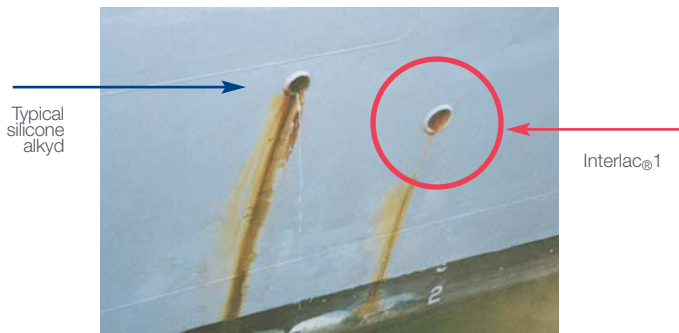
Rust stain hiding after 10 months in service
