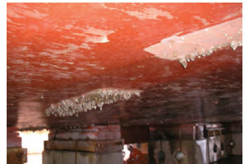
Seismic research vessel after 44 months in the Gulf of Mexico showing excellent antifouling performance
