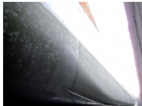
Intersleek 900 test patch on VLCC after 59 months
