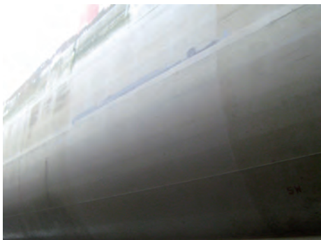
Intersleek 900 test patch on LNG after 30 months
