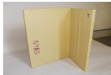
Interline 994LT after 14 months and 20 cargo sequences: Test panels present no defects.
