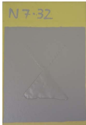
Detachment of topcoat following use of unapproved pen
