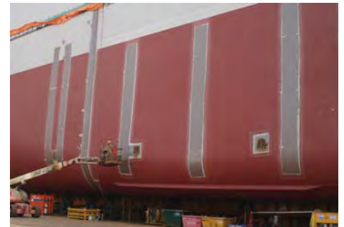
Newbuilding application to erection joints on an underwater hull
