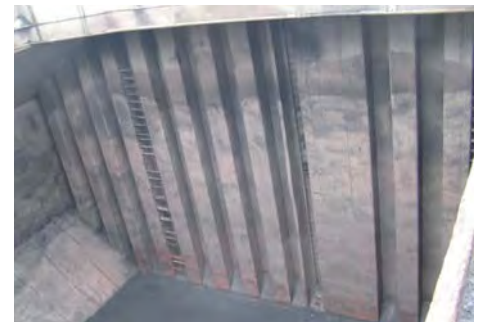
Intergard®7600 after 6 months in service on a 40k dwt bulk carrier
