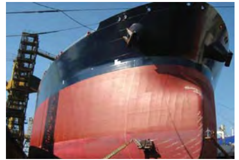
In-dock condition after HPFWW
